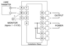
Note: Use shielded cables for I/O wiring.
