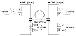
\*Input shunt resistor attached for current input.
