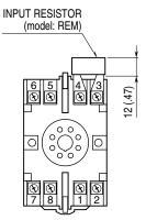
Input shunt resistor attached for current input.
