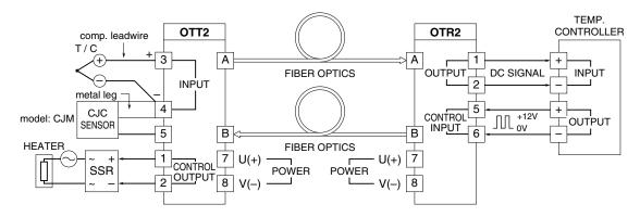
The OTT2 unit converts mV input signals from a thermocouple into light pulse reflections, and transmits them to the OTR2 unit via fiber optics cable (A), while the OTR2 converts the light pulse reflections into analog signals and output them to a temperature controller.
