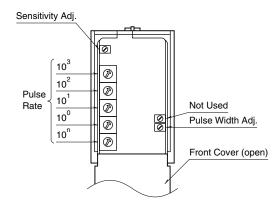
• **Pulse rate adjustment**: switches are assigned as shown in the equation below.
