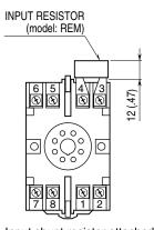
Input shunt resistor attached for current input.
