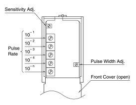
Positions for the rotary switches  $10^{-1}$  through  $10^{-n}$  apply respectively to each digit of the decimals and exponential as shown below.
