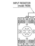
Input shunt resistor attached for current input.
