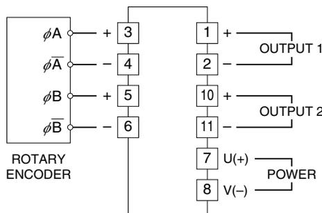
Note 1: Sensor excitation not provided for RS-422 line driver pulse input.
