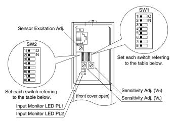
There is no need of hardware adjustment for RS-422 line driver pulse input. Unnecessary switches or LEDs are not provided.
