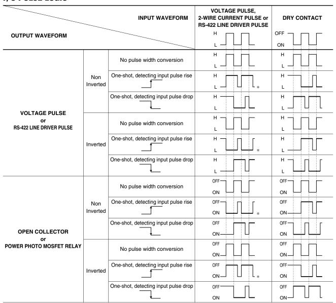
The pulse width in one-shot means the bold lined section of a pulse waveform.
