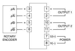
Note 1: Sensor excitation not provided for RS-422 line driver pulse input. Note 2: Not negative common in case of RS-422 line driver pulse output or power photo MOSFET relay output.
