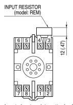
Input shunt resistor attached for current input.
