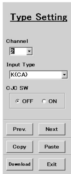
The image shows a 'Type Setting' dialog box. At the top, the title 'Type Setting' is underlined. Below it, there are three sections: 'Channel' with a pull-down menu showing '2', 'Input Type' with a pull-down menu showing 'K(CA)', and 'C.JC SW' with two radio buttons, 'OFF' and 'ON', where 'OFF' is selected. At the bottom, there are two rows of buttons: the first row has 'Prev.' and 'Next'; the second row has 'Copy' and 'Paste'; the third row has 'Download' and 'Exit'.
