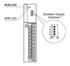
\*1. Excitation supply switches 1 through 4 turn on (ON) or off (OFF) the power supply to the input 1 through 4 respectively. (Factory set to ON)
