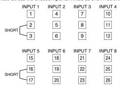
The input will become unstable if unused channels are left open. Unused channels can be specified and set so on the PC Configurator Software (model: R3CON) without needing to short at the field terminals.
