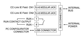
Regarding CN1 and CN2 of RJ-45 connector for CC-Link IE Field network, there is no restriction for connection order.
