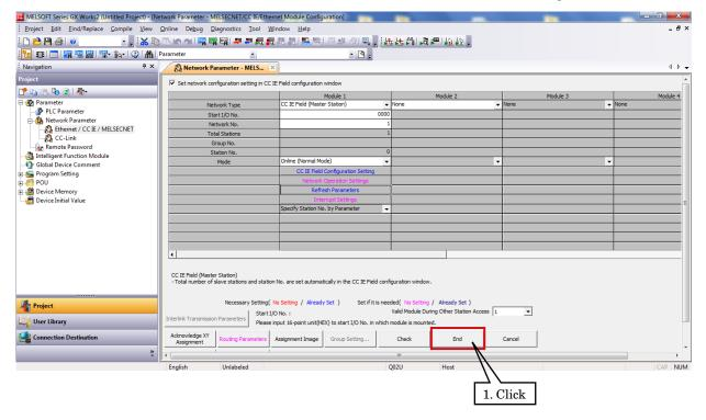
8) After creating a program as necessary, write the parameter and the program to the CPU unit.
