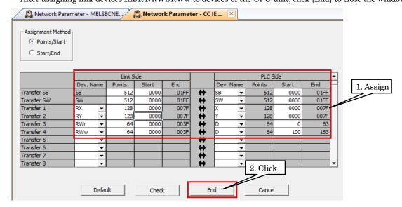
7) Click [End] to close the [Network Parameter – MELSECNET/CC IE Ethernet Module Configuration] window.
