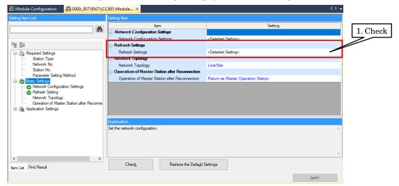
After assigning link devices RX/RY/RWr/RWw to devices of the CPU module, click [Apply] to close the window.
