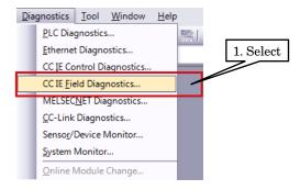
2) Click the station to be diagnosed so that the station status is displayed on the [Selected Station Communication Status Monitor].
