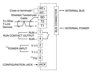
\* When the module is at an end of the transmission line via twisted-pair cable (= when there is no cross wiring), close across the RT+ and RT- terminals with the jumper included in the product package. Remove the jumper for all other locations. \*\*Not provided with 'No Power Supply' type module. Caution: FG terminal is NOT a protective conductor terminal.
