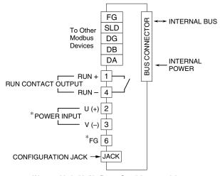
\*Not provided with 'No Power Supply' type module. Caution: FG terminal is NOT a protective conductor terminal.
