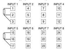
Unused channels left open are equal to the burnout, which turns the red ERR LED on and sets a burnout flag at the PLC or the host
