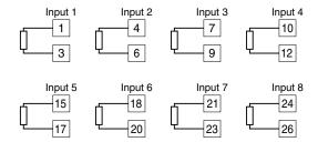
Unused channels left open are equal to the burnout, which turns the red ERR LED on and sets a burnout flag at the PLC or the host device.
