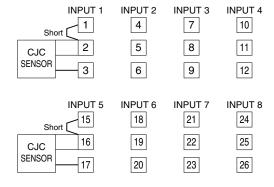
Unused channels left open are equal to the burnout, which turns the red ERR LED on and sets a burnout flag at the PLC or the host device.
