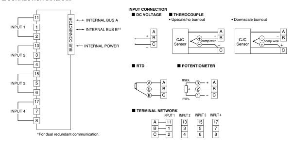
Note 1: Remove CJC sensor for RTD or potentiometer input. The CJC sensor does not affect to DC voltage input.
