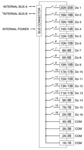
Numbers in italic indicate LED No.s assigned to the front panel LEDs. \*For dual redundant communication.
