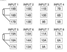
Unused channels left open are equal to the burnout, which turns the red ERR LED on and sets a burnout flag at the PLC or the host device.
