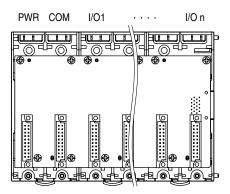
3) Tighten the base fixing screw using a screwdriver (stem length: 70 mm/2.76" or more) (torque 0.5 N·m).
