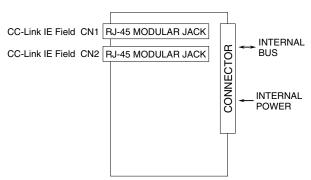
CN1 and CN2 of RJ-45 modular jacks for CC-Link IE Field network can be connected in any order.
