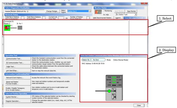
3) If an error has occurred, the button such as [Module Error] is displayed. Click the button to display the details, and troubleshoot accordingly.
