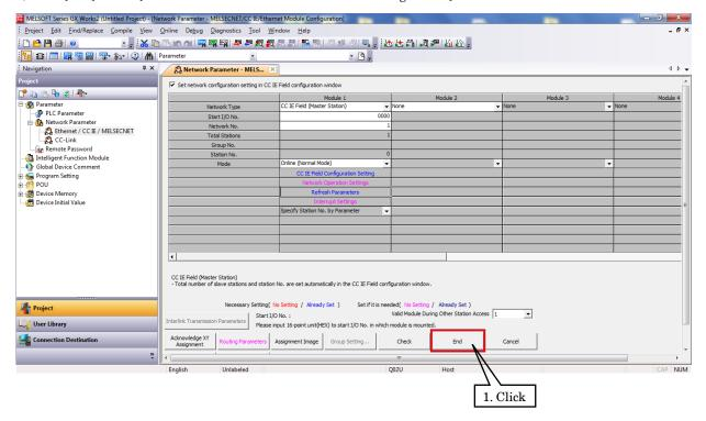
8) After having programmed as necessary, write parameters and programs to CPU unit.
