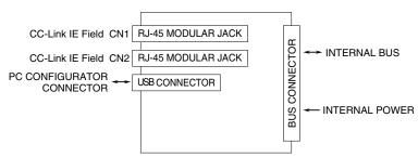
Regarding CN1 and CN2 of RJ-45 connector for CC-Link IE Field network, there is no restriction for connection order.
