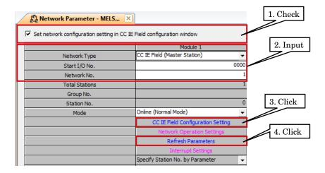
5) Click [CC IE Field Configuration Setting] to open the window of configuration setting.
