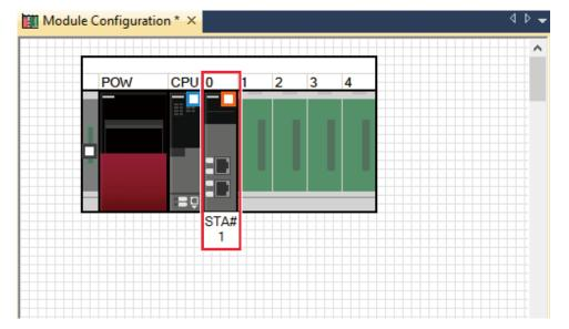
7) Set Station Type to [Master Station], Network No. to 1 in [Required Settings].
