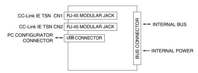
Regarding CN1 and CN2 of RJ-45 connector for CC-Link IE TSN network, there is no restriction for connection order.
