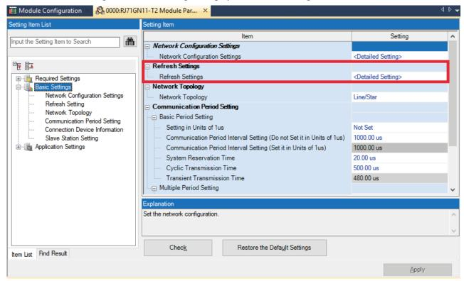
Assign link devices RX/RY/RWr/RWw to devices of the CPU unit, click [Apply] to close the window.
