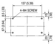
\*Working space required for mounting/unmounting the modules.
