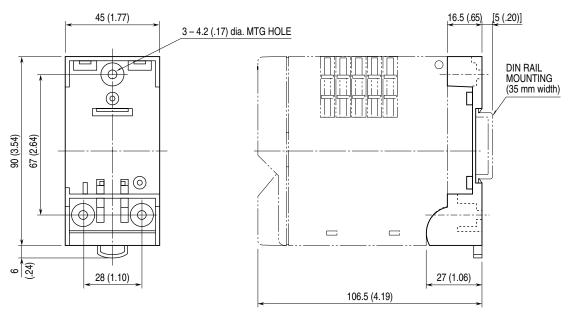
Use an end bracket to secure the connection of the extender base on a DIN rail.
