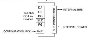
Note: The FG terminal is not connected with the FG of the power supply module (model: R5-PS).
