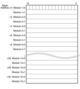
The area enclosed with a bold line is assigned for I/O data.
