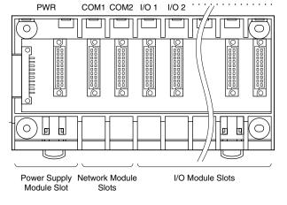
The Network Interface Modules must be mounted on the COM1 on the Base.
