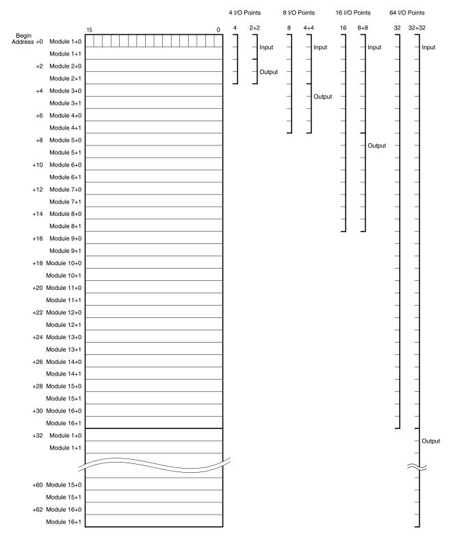
Total number of I/O modules are half the assigned I/O points with Data Allocation Mode 2. I/O modules can be allocated from I/O Module Slot No. 1.
