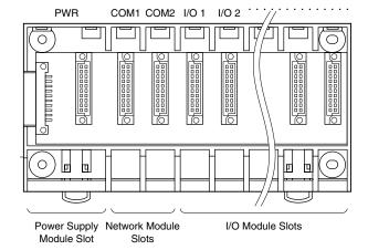
The Network Interface Module must be mounted on the COM1/COM2 on the Base.
