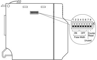
Counter Reset SW is normally OFF during operation.
