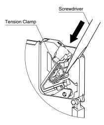
2) Insert a wire. Push the screwdriver toward the direction indicated with the arrow in the figure below to widen the opening if necessary.
