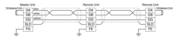
Be sure to connect the terminating resistor across DA and DB at both ends of communication line. When this unit is located at an end, turn the terminating resistor SW ON. The Master Unit can be located at not only both ends but also any node of the of communication line.
