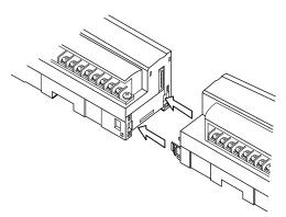
3) Mount the combined module on a DIN rail.
