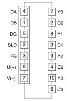
Caution: FG terminal is NOT a protective conductor terminal.
