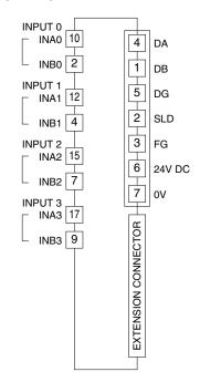
Caution: FG terminal is NOT a protective conductor terminal.
