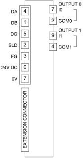
In order to improve EMC performance, bond the FG terminal to ground. Caution: FG terminal is NOT a protective conductor terminal.
