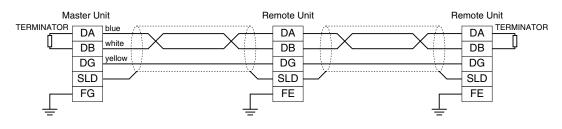
Be sure to connect the terminating resistor across DA and DB at both ends of communication line. When this unit is located at an end, turn the terminating resistor SW ON. The Master Unit can be located at not only both ends but also any node of the of communication line.
