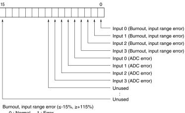
0 : Normal 1 : Error ADC error (no response from ADC)
