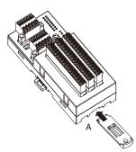
B)Set the upper hook at the rear side of the unit on the DIN rail.
