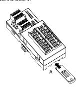
B)Set the upper hook at the rear side of the unit on the DIN rail.
