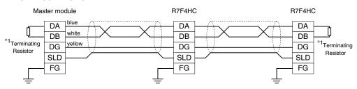
\*1. Turn on the terminator DIP switch to activate the internal terminating resistor.
