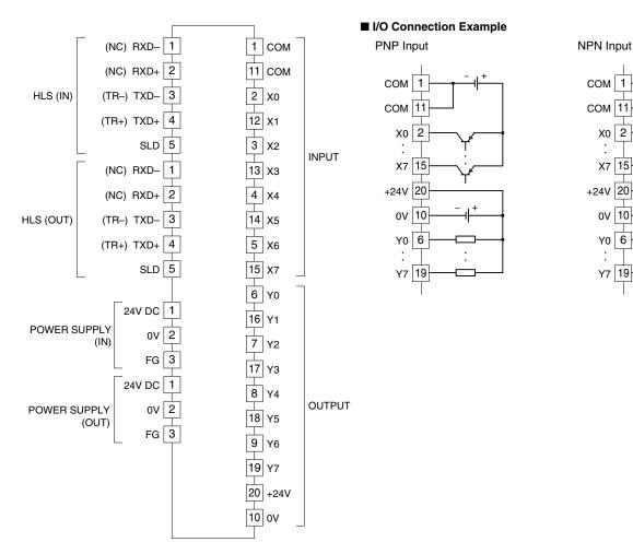
Note 1: Terminal numbers in parentheses are for half-duplex communication model. Note 2: In order to improve EMC performance, bond the FG terminal to ground. Caution: FG terminal is NOT a protective conductor terminal.
