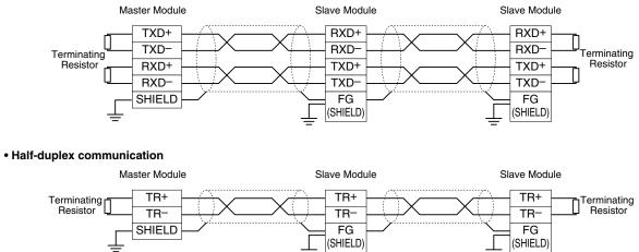
Note: Be sure to turn ON the switch of the terminating resistor located at both ends of the modules.
