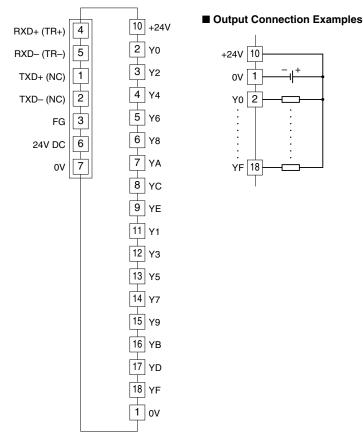
Note 1: Terminal numbers in parentheses are for half-duplex communication model. Note 2: In order to improve EMC performance, bond the FG terminal to ground. Caution: FG terminal is NOT a protective conductor terminal.
