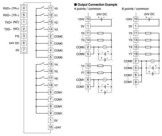
Note 1: Terminal numbers in parentheses are for half-duplex communication model. Note 2: In order to improve EMC performance, bond the FG terminal to ground. Caution: FG terminal is NOT a protective conductor terminal.
