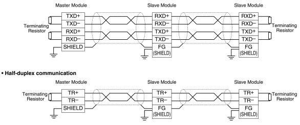
Note: Be sure to turn ON the switch of the terminating resistor located at both ends of the modules.
