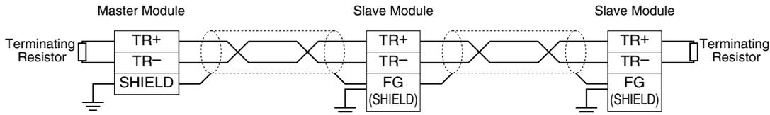
Note: Be sure to turn ON the switch of the terminating resistor located at both ends of the modules.
