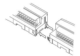
3) Mount the combined module on a DIN rail.
