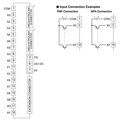
\*MECHATROLINK connectors are internally connected. The network cable can be connected to either one.
